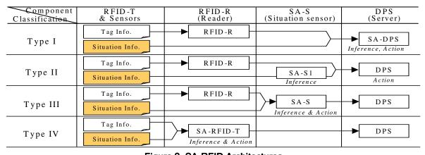
Figure 2. SA-RFID Architectures
