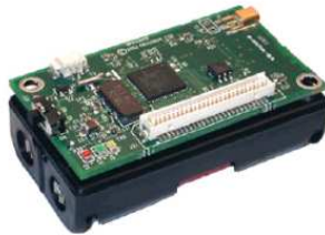
Figure 3.1: Mica2 wireless sensor node.
