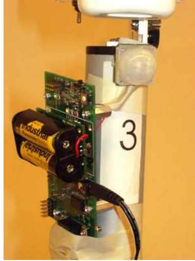
Figure 7.1: PIR sensor and programmer connected to a post.
