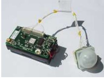
Figure 4.1: Mica2 node with a PIR sensor connected to it.
