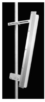
The TA-2304-2-45-ISM is a vertically polarized sectoral antenna with a fixed 45 degree pattern. The antenna consists of a printed dipole array enclosed in an aluminum base with a UV stabilized radome for superior weatherability. It is designed for wireless data in the ISM band and is at DC ground to aid in lightning protection.
