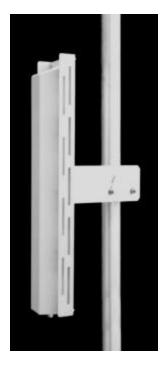
The TA-2405H-4-60 is a horizontally polarized 60 degree sectoral antenna. It was designed specifically for wireless data and point-to-multipoint radio applications. Radiating elements are protected by a weatherproof radome for operation under severe weather conditions (icing, salt air, acid rain, etc.) and are at DC ground to aid in lightning protection.
