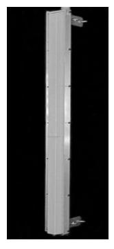
The TA-2304-4-ISM is a vertically polarized high gain sectoral antenna which can be ordered with adjustable side panels for 60 - 160 degree patterns. The antenna consists of a printed dipole array enclosed in an aluminum base with a UV stabilized radome for superior weatherability. The antenna is at DC ground to aid in lightning protection. Due to the very narrow elevation beamwidth, TIL-TEK recommends that this antenna be used on stable platforms and where other options are not practical.
