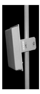
The TA-2408 is a vertically or horizontally polarized panel antenna. The antenna consists of a printed broadband dipole array enclosed in an aluminum cavity with a UV stabilized ASA radome for superior weatherability. It is designed for wireless data in the ISM band and is at DC ground to aid in lightning protection.
