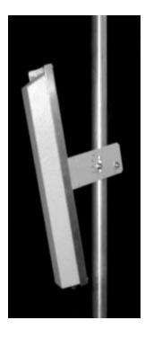
The TA-2404-4-90 is a vertically polarized 90 degree sectoral antenna. It was designed specifically for wireless data and point-to-multipoint radio applications. Radiating elements are protected by a weatherproof radome for operation under severe weather conditions (icing, salt air, acid rain, etc.) and are at DC ground to aid in lightning protection.
