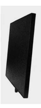
The TA-2407P is a compact, light-weight, vertically polarized panel antenna intended for mounting onto the back of a laptop computer for special applications in the ISM band. The antenna consists of a printed patch array enclosed in a black painted aluminum cavity with a black UV stabilized ASA radome.
