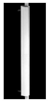
The TA-2304-4-180-ISM is a vertically polarized high gain 180 degree sectoral antenna. The antenna consists of a printed dipole array enclosed in an aluminum base with a UV stabilized radome for superior weatherability. The antenna is at DC ground to aid in lightning protection. Due to the very narrow elevation beamwidth, TIL-TEK recommends that this antenna be used on stable platforms and where other options are not practical.
