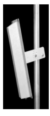
The TA-2405H-4-90 is a horizontally polarized 90 degree sectoral antenna. It was designed specifically for wireless data and point-to-multipoint radio applications. Radiating elements are protected by a weatherproof radome for operation under severe weather conditions (icing, salt air, acid rain, etc.) and are at DC ground to aid in lightning protection.
