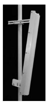
The TA-2304-2-ISM is a vertically polarized sectoral antenna which has adjustable side panels for 60-160 degree azimuth patterns. The antenna consists of a printed dipole array enclosed in an aluminum base with a UV stabilized radome for superior weatherability. It is designed for wireless data in the ISM band and is at DC ground to aid in lightning protection.
