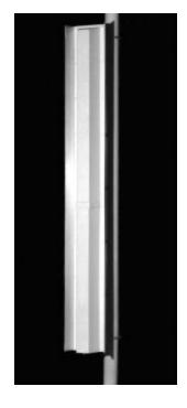
The TA-2304-4-45-ISM is a vertically polarized high gain 45 degree sectoral antenna. The antenna consists of a printed dipole array enclosed in an aluminumun base with a UV stabilized radome for superior weatherability. The antenna is at DC ground to aid in lightning protection. Due to the very narrow elevation beamwidth, TIL-TEK recommends that this antenna be used on stable platforms and where other options are not practical.
