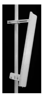
The TA-2304-2-180-ISM is a vertically polarized sectoral antenna with a fixed 180 degree pattern. The antenna consists of a printed dipole array enclosed in an aluminum base with a UV stabilized radome for superior weatherability. It is designed for wireless data in the ISM band and is at DC ground to aid in lightning protection.
