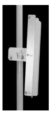
The TA-2304-ISM is a vertically polarized sectoral antenna which has adjustable side panels for 60-160 degree azimuth patterns. The antenna consists of a printed dipole array enclosed in an aluminum base with a UV stabilized radome for superior weatherability. It is designed for wireless data in the ISM band and is at DC ground to aid in lightning protection.
