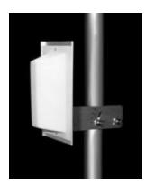
The TA-2404-2-90 is a vertically polarized 90 degree sectoral antenna. It was designed specifically for wireless data and point-to-multipoint radio applications. Radiating elements are protected by a weatherproof radome for operation under severe weather conditions (icing, salt, air, acid rain, etc.) and are at DC ground to aid in lightning protection.
