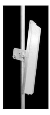
The TA-2304-180-ISM is a vertically polarized sectoral antenna with a fixed 180 degree pattern. The antenna consists of a printed dipole array enclosed in an aluminum base with a UV stabilized radome for superior weatherability. It is designed for wireless data in the ISM band and is at DC ground to aid in lightning protection.
