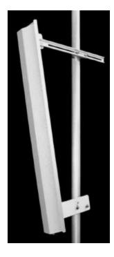
The TA-2404-8-120 is a vertically polarized 120 degree sectoral antenna. It was designed specifically for wireless data and point-to-multipoint radio applications. Radiating elements are protected by a weatherproof radome for operation under severe weather conditions (icing, salt air, acid rain, etc.) and are at DC ground to aid in lightning protection.
