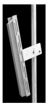
The TA-2404-4-60 is a vertically polarized 60 degree sectoral antenna. It was designed specifically for wireless data and point-to-multipoint radio applications. Radiating elements are protected by a weatherproof radome for operation under severe weather conditions (icing, salt air, acid rain, etc.) and are at DC ground to aid in lightning protection.
