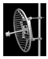
The TA-2436 is a grid parabolic antenna with a broadband dipole horn feed which is sealed for superior weatherability. The antenna is at DC ground to aid in lightning protection. This antenna is extremely rugged and is designed to provide superior performance in any conditions.
